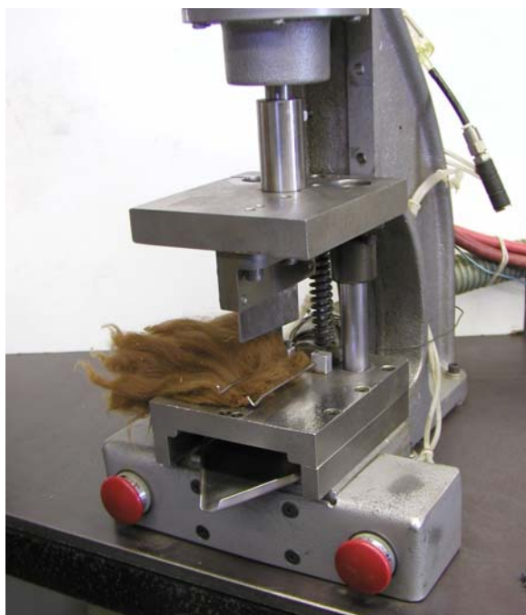
Figure 5. Fiber sample positioned in the die cutter to permit 2-mm snippets at base of staple.
