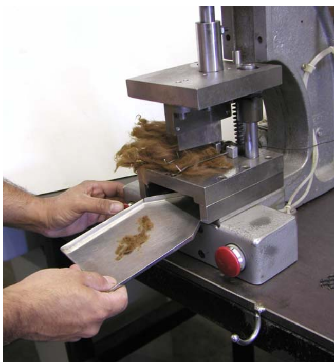
Figure 6. 2-mm die cut samples in collection tray. Typically, several thousand individual fibers are collected.
